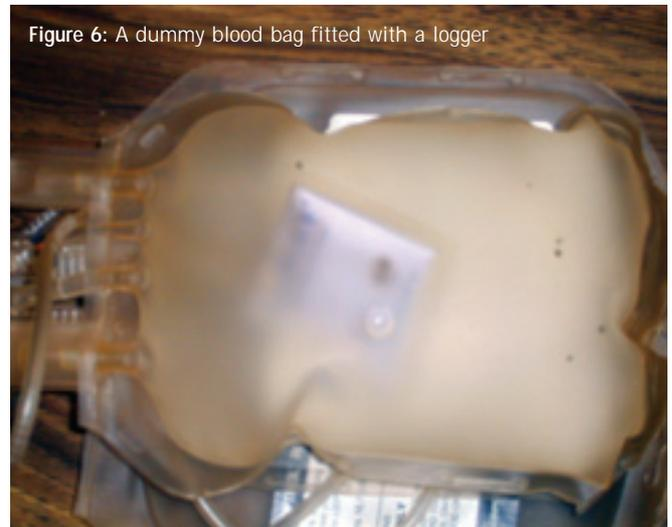
Figure 6: A dummy blood bag fitted with a logger
