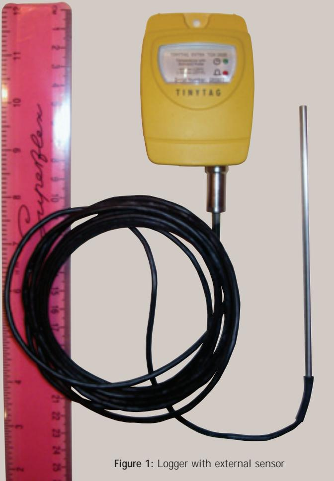
Figure 1: Logger with external sensor
