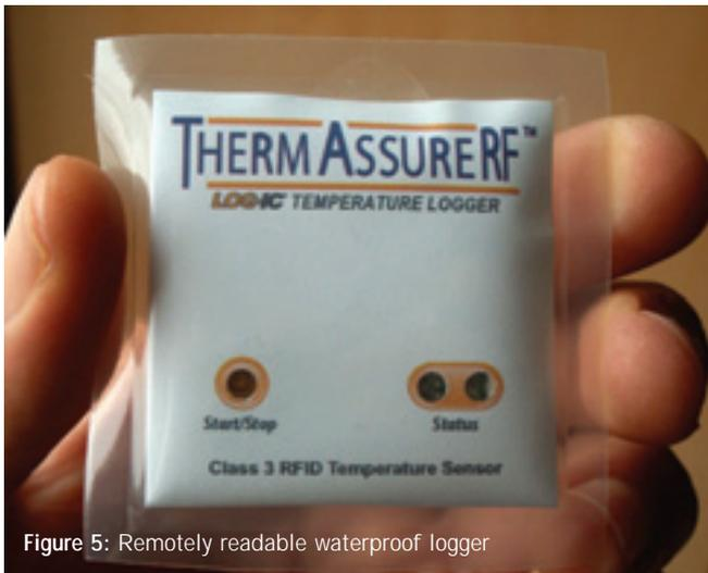
Figure 5: Remotely readable waterproof logger
