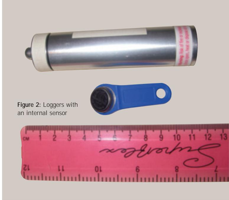
Figure 2: Loggers with an internal sensor
