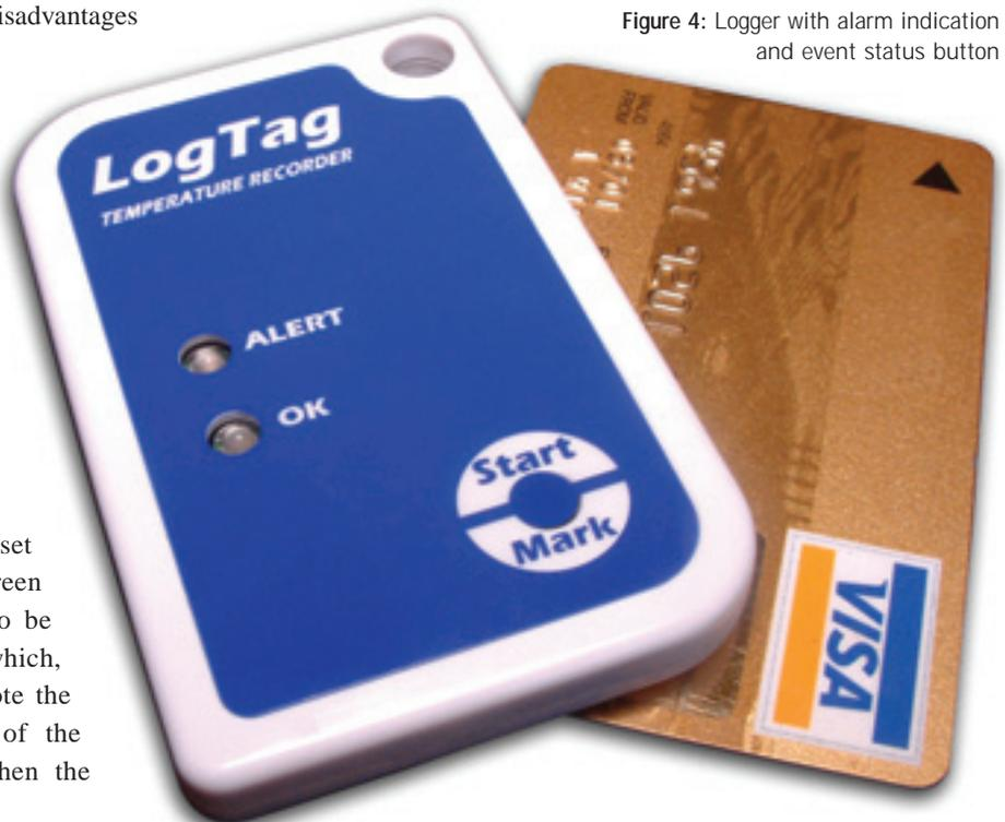
Figure 4: Logger with alarm indication and event status button
